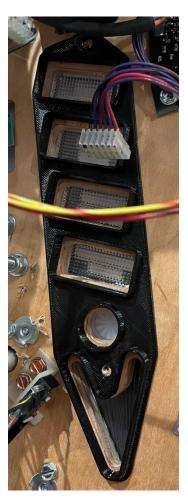
For the city baffle you will need to unscrew the factory flasher bulb socket and retain the screw. The new white cone has a lip that will help keep the cone centered on the insert opening. Use the new supplied longer hex head screw that was temporally installed in the cone to secure the cone to the playfield. The factory shorter screw that you just removed from the lamp socket is to be used to hold the socket to the new mount on the cone body. Do not overtighten!
