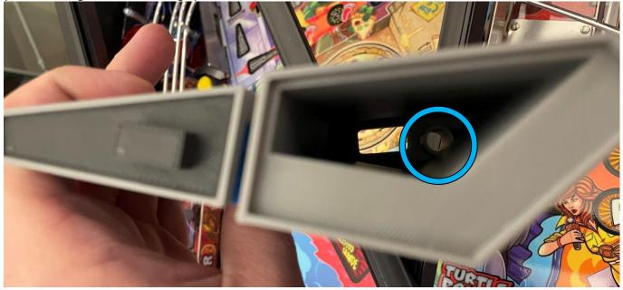
Take the screw and washer from step 4 and place it on the tip of the screwdriver inverted as shown below.
