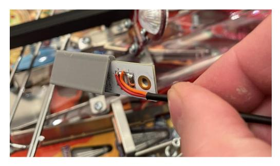
After the board is pushed all the way in it should look like this from the front of the wedge. The LED is facing out.
